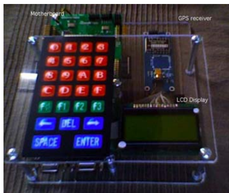
Fig. 10 First version of the prototype of the data logger that is being developed for the verification of taximeters. An evolution of this device is shown in Fig. 11
